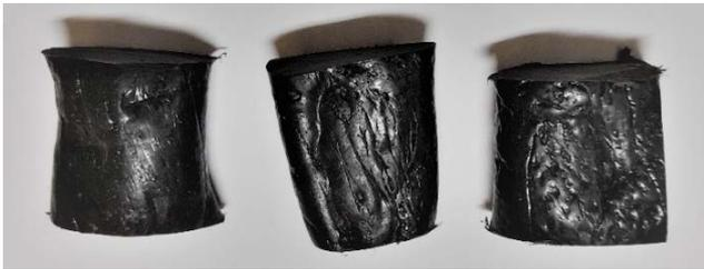
**Fig. 4.** Plastic aggregate particle for compression testing
