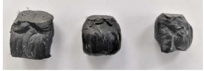
**Fig. 5.** Tested plastic aggregate particle under compression
