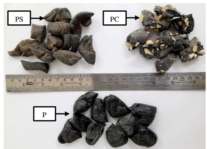
Fig. 3. Picture of proposed plastic aggregates
