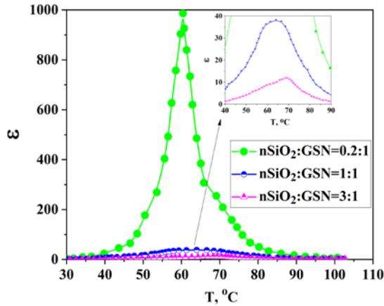
**Fig. 3.** The results for phase transition testing for composite samples containing different nSiO<sub>2</sub> content
