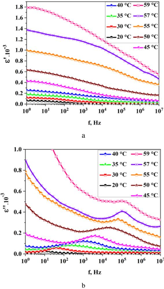
**Fig. 5.** Frequency dependences of dielectric permittivity at different temperatures under phase transition point for the composite samples of  $n\text{SiO}_2:\text{GSN} = 0.2:1$ : a – real parts; b – imaginary parts
