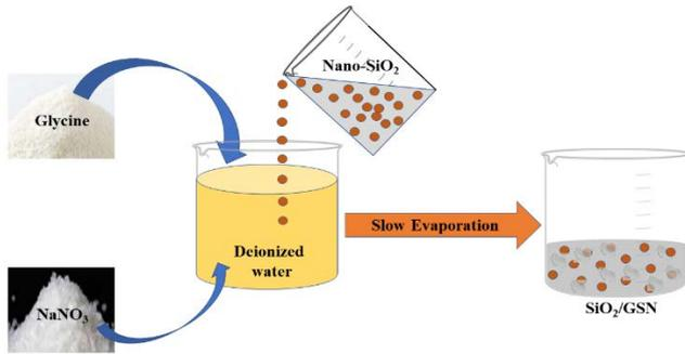
**Fig. 1.** Scheme for preparation of nSiO<sub>2</sub>/GSN nanocomposite
