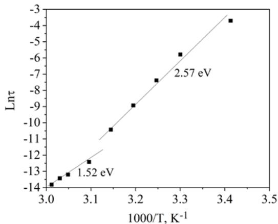
**Fig. 6.** Inverse temperature dependences of relaxation time at different temperatures under phase transition point for the composite samples of  $n\text{SiO}_2:\text{GSN} = 0.2:1$
