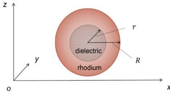
**Fig. 1.** The structure of the spherical nanoshell consisting of rhodium and dielectric. The radius of the dielectric core is labeled in  $r$  and the radius of the rhodium nanoshell is indicated in  $R$
