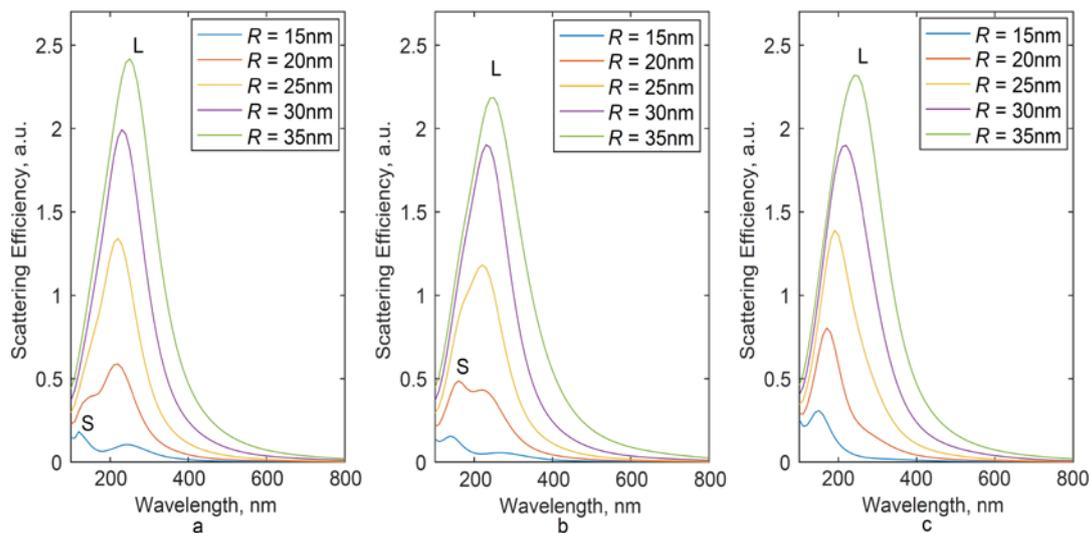
**Fig. 2.** Scattering efficiency as a function of incident light's wavelength. The dielectric material in the core was a– $\text{SiO}_2$ ; b– $\text{Si}_3\text{N}_4$ ; c– $\text{TiO}_2$ . The radius of the core was fixed to be  $r = 10$  nm
