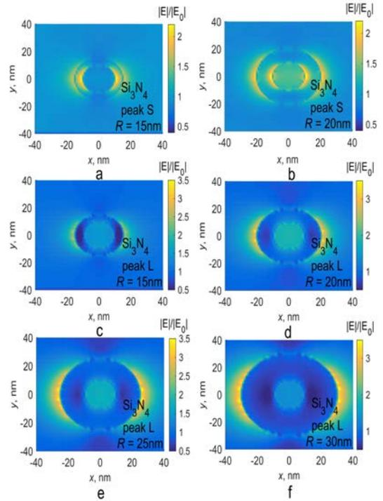
**Fig. 4.** Electric field distribution in the  $x$ - $y$  plane for the case shown in Fig. 2 b. The nanoshell radius  $R$ : a, c–15 nm; b, d–20 nm; e–25 nm; f–30 nm. The wavelength correlates to a and b peak S, and c–f peak L. Note that the maximum intensity of the color bar is not the same
