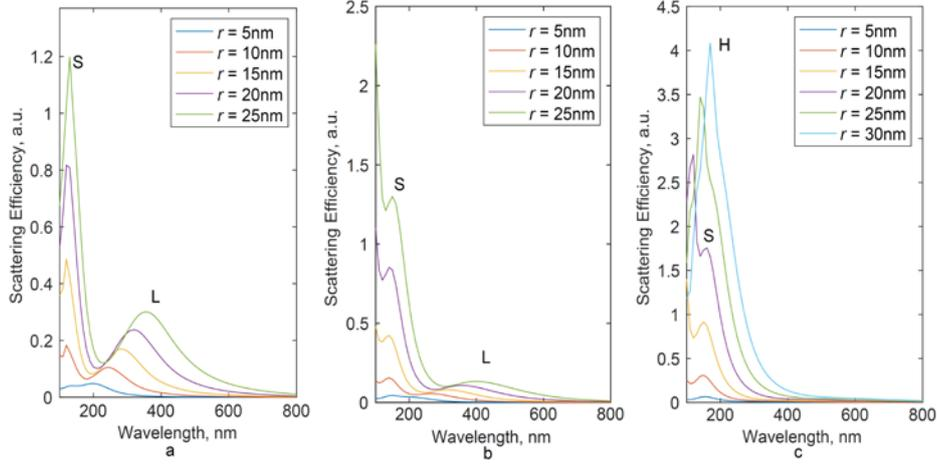
**Fig. 6.** Scattering efficiency as a function of incident light's wavelength. The dielectric material in the core: a –  $\text{SiO}_2$ ; b –  $\text{Si}_3\text{N}_4$ ; c –  $\text{TiO}_2$ . The thickness of the rhodium nanoshell was fixed to be  $R - r = 5$  nm
