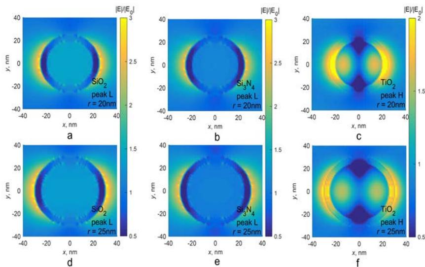
**Fig. 8.** Electric field distribution in the  $x$ - $y$  plane for the case shown in Fig. 6. The dielectric core: a, d –  $\text{SiO}_2$ ; b, e –  $\text{Si}_3\text{N}_4$ ; c, f –  $\text{TiO}_2$ . The radius of the core: a, b, c – 20 nm; d, e, f – 25 nm. The wavelength correlates to a and d peak L in Fig. 6 a; b and e peak L in Fig. 6 b; c and f peak H in Fig. 6 c. Note that the maximum intensity of the color bar is not the same
