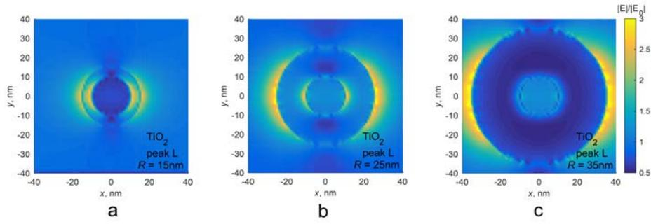
**Fig. 5.** Electric field distribution in the  $x$ - $y$  plane for the case shown in Fig. 2 c. The nanoshell radius  $R$ : a – 15 nm; b – 25 nm; c – 35 nm. The wavelength correlates to the single peak
