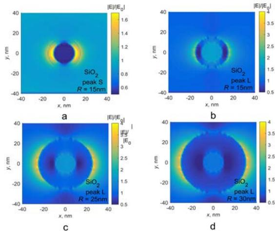
**Fig. 3.** Electric field distribution in the  $x$ - $y$  plane for the case shown in Fig. 2 a. The nanoshell radius  $R$ : a, b–15 nm; c–25 nm; d–30 nm. The wavelength correlates to a peak S, and b, c, d peak L. Note that the maximum intensity of the color bar is not the same
