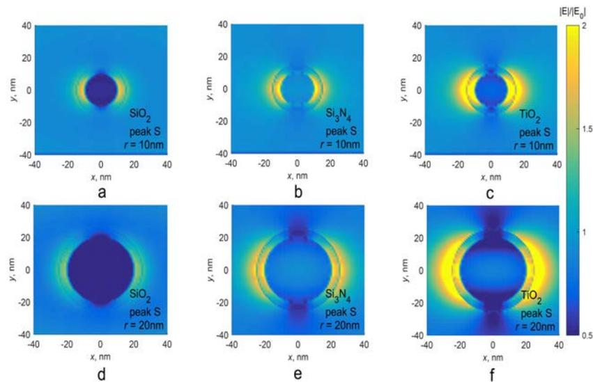
**Fig. 7.** Electric field distribution in the  $x$ - $y$  plane for the case shown in Fig. 6. The dielectric core: a, d –  $\text{SiO}_2$ ; b, e –  $\text{Si}_3\text{N}_4$ ; c, f –  $\text{TiO}_2$ . The radius of the core: a, b, c – 10 nm; d, e, f – 20 nm. All the wavelengths correlate to peak S indicated in Fig. 6
