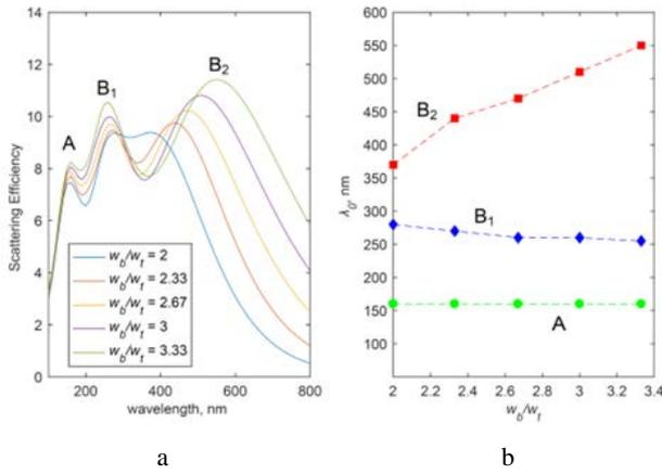
**Fig. 4.** a–scattering efficiency as a function of wavelength at different width ratios of bottom bar to top bar; b–resonance wavelength ( $\lambda_0$ ) as a function of the width ratio. In the simulations  $w_t = 30$  nm and  $h = 50$  nm.  $w_b$  was varied from 60 to 100 nm so that  $w_b/w_t$  was changed from 2 to 3.33. The incident light was  $x$ -polarized
