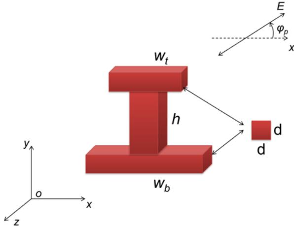
**Fig. 1.** The structure of the I-shaped nanomaterial consisting of rhodium. The width of the top bar is  $w_t$ , the width of the bottom bar is  $w_b$ , and the height of the post is  $h$ . The cross sections of the bars and the post are all squared, with a fixed area of  $d \times d$ . The polarization of incident light is expressed by  $\varphi_p$ , which is the angle between the electric vector and the  $x$ -axis
