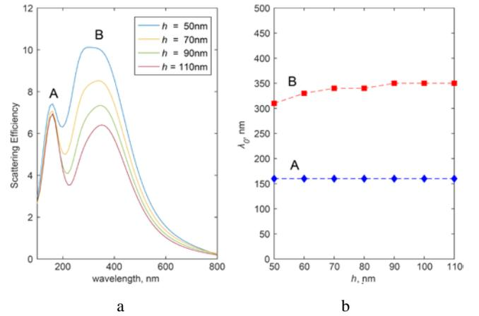
**Fig. 2.** a—scattering efficiency as a function of wavelength at different heights of the post; b—resonance wavelength ( $\lambda_0$ ) as a function of the height. In the simulations  $w_t = 30 \text{ nm}$  and  $w_b = 50 \text{ nm}$ . The incident light was  $x$ -polarized
