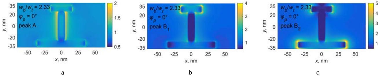
**Fig. 5.** Electric field distribution in the  $x$ - $y$  plane with  $w_b/w_t = 2.33$ : a–peak A; b–peak B<sub>1</sub>; c–peak B<sub>2</sub>
