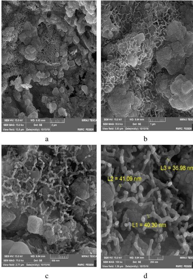
Fig. 5. FESEM of coated electroless of Ni–P–0.1g/l Fe<sub>2</sub>O<sub>3</sub> and annealed: a–2 μm; b–1 μm; c–500 nm; d–200 nm magnification
