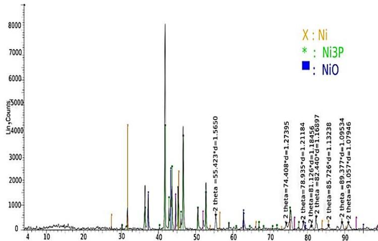
Fig. 7. X-ray diffraction patterns of annealed Ni-P-0.1 g/L Fe<sub>2</sub>O<sub>3</sub> sample
