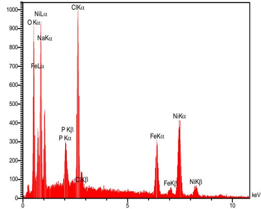
Fig. 6. Analysis of EDX for the surface of Ni–P–Fe<sub>2</sub>O<sub>3</sub> coating
