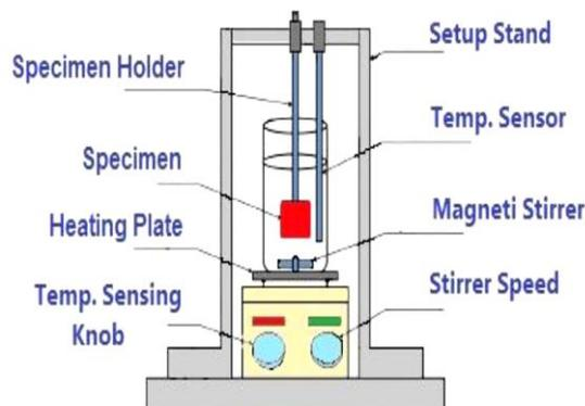
**Fig.1.** Experimental setup for the electroless deposition process
