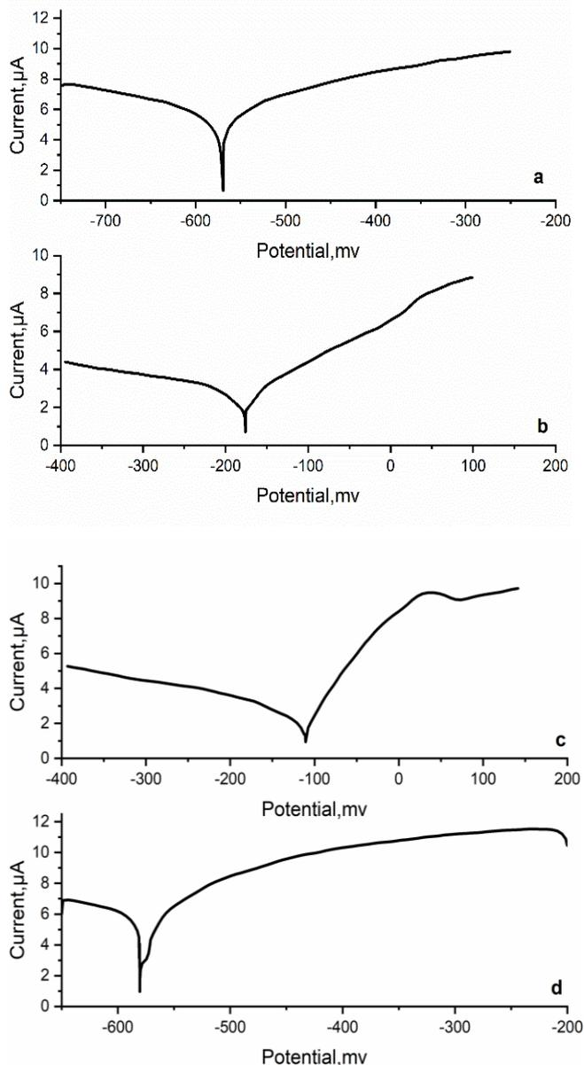
**Fig. 10.** Polarization of Tafel curves: a – as-substrate; b – Ni–P; c – Ni–P–0.1 g/l Fe<sub>2</sub>O<sub>3</sub>; d – Ni–P–0.3 g/l Fe<sub>2</sub>O<sub>3</sub> annealed samples
