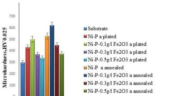
Fig. 8. Microhardness of plated and annealed specimen's surface
