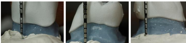
Fig. 4. Macroscopic analysis of the marginal fit of Custom orientation crowns. The “frosty” look of the surface is caused by the scanning powder used
