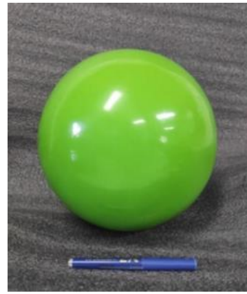
Fig. 9. 3D printed spherical float manufactured by FDM process
