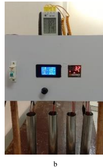
Fig. 1. The apparatus for operation evaluation of LHSM as LTES: a – schematic; b – photograph
