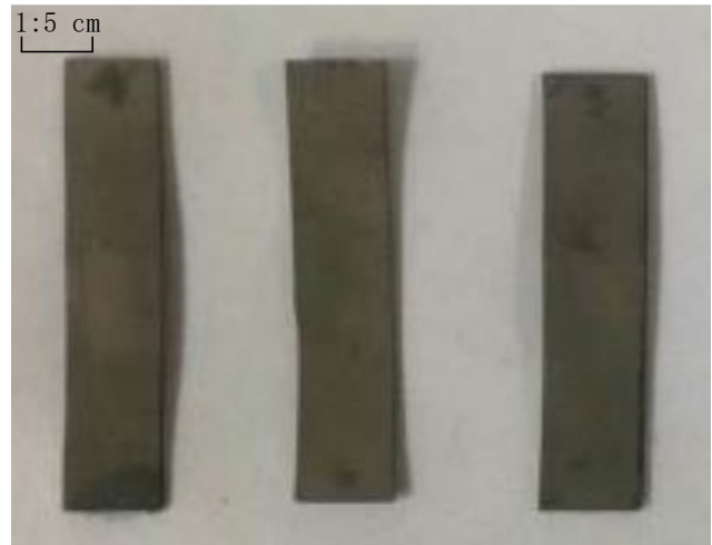
Fig. 6. Physical image of IPMC thin film
