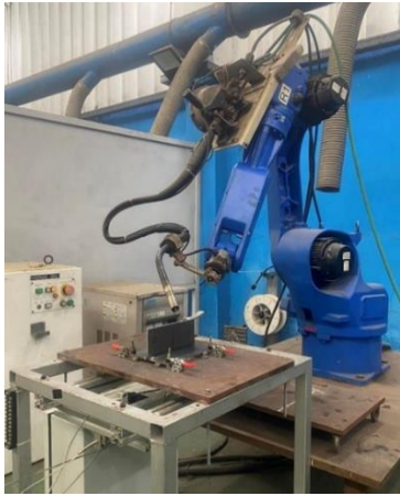
Fig. 5. The overall setup: welding system with the 6DOF robot arm and welding table
