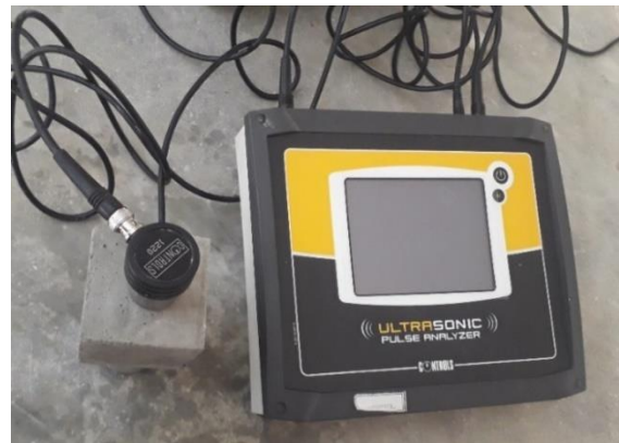
Fig. 8. Apparatus used for ultrasonic pulse velocity
