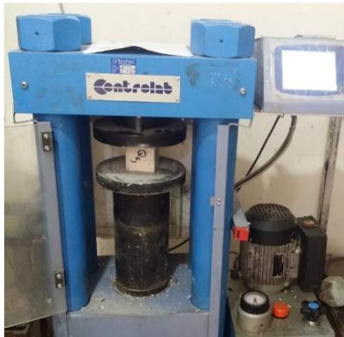
Fig. 6. Test specimens prior to compression testing
