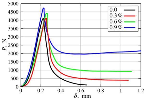
**Fig. 4.** Load  $P$  versus deflection  $\delta$  curves for concrete with various volume fraction of fibres type A
