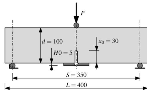
Fig. 2. Fracture testing configuration and geometry of specimen
