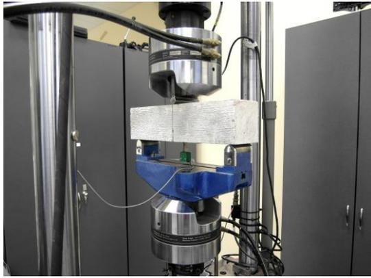
Fig. 3. Notched beam specimen during testing
