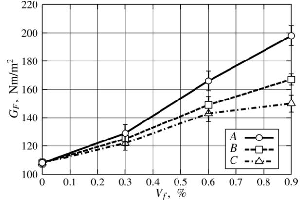
**Fig. 7.** Effect of fibre type and volume fraction  $V_f$  (%) on fracture energy  $G_F$  calculated for deflection  $\delta=0.70$  (vertical bars represent the range of accuracy)
