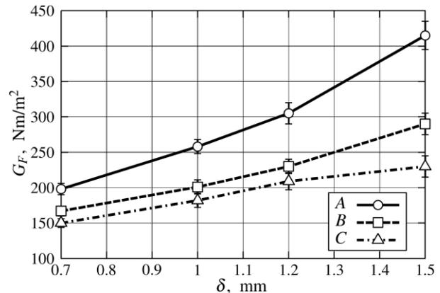
**Fig. 8.** Dissipated energy  $G_F$  versus  $\delta$  for concretes with different type of fibres ( $V_f=0.9\%$ ) (vertical bars represent the range of accuracy)
