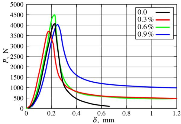
**Fig. 5.** Load  $P$  versus deflection  $\delta$  curves for concrete with various volume fraction of fibres type B
