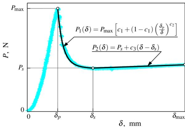
Fig. 9. Equations for experimental curve fitting
