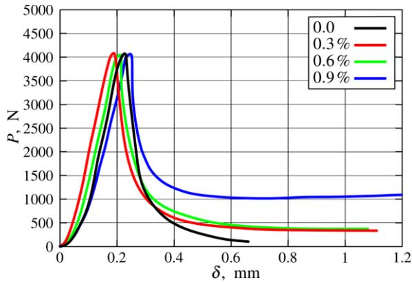
**Fig. 6.** Load  $P$  versus deflection  $\delta$  curves for concrete with various volume fraction of fibres type C
