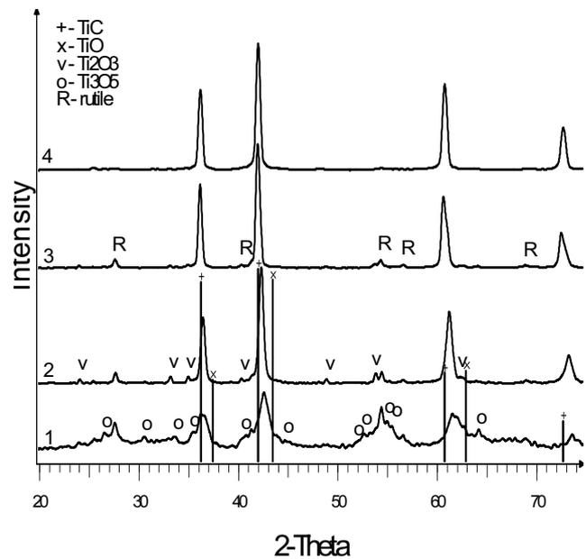
**Fig. 1.** The dependence of phase composition of A series samples on the temperature of thermal treatment: 800 °C (1); 1000 °C (2); 1200 °C (3) and 1360 °C (4)
