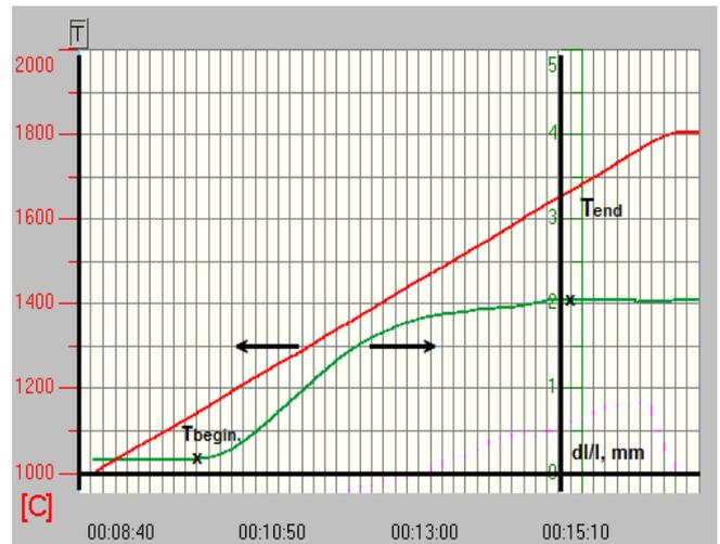
**Fig. 5.** Fragment of the shrinkage curve of titanium carbide in the range from 1000 °C to 1800 °C at the SPS process
