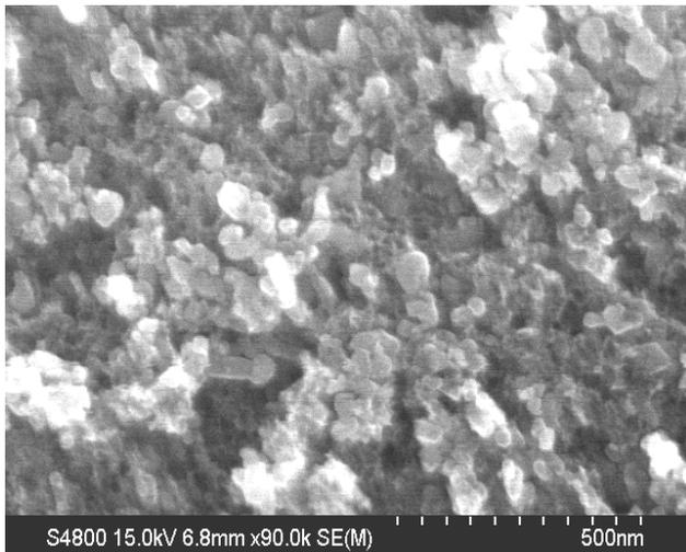
**Fig. 4.** Micrographs of B series nanopowders obtained at 1400 °C 1 h
