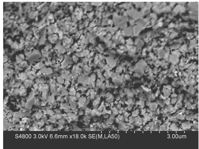
**Fig. 6.** Microstructure of the sample of TiC compacted at 1800 °C by SPS
