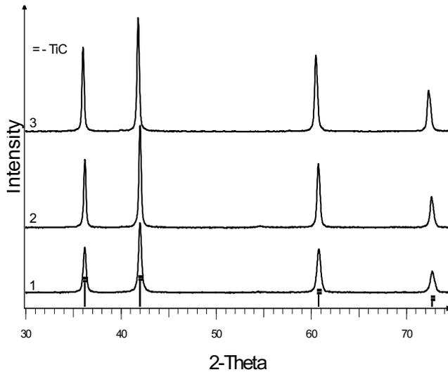
**Fig. 3.** The dependence of phase composition of B series samples on the temperature of thermal treatment: 1350 °C, 1 h (1); 1350 °C, 2 h (2) and 1400 °C, 1 h (3)
