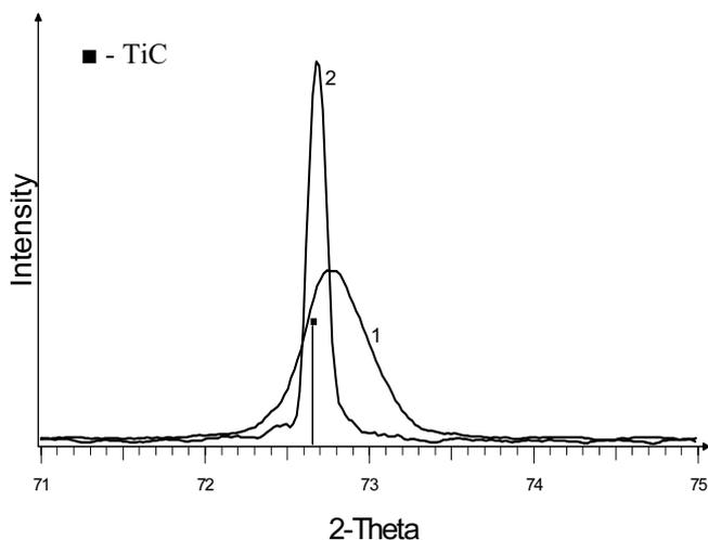
**Fig. 7.** Fragment of the phase composition of TiC nanopowder (1) and sample of TiC compacted at 1800 °C by SPS (2)
