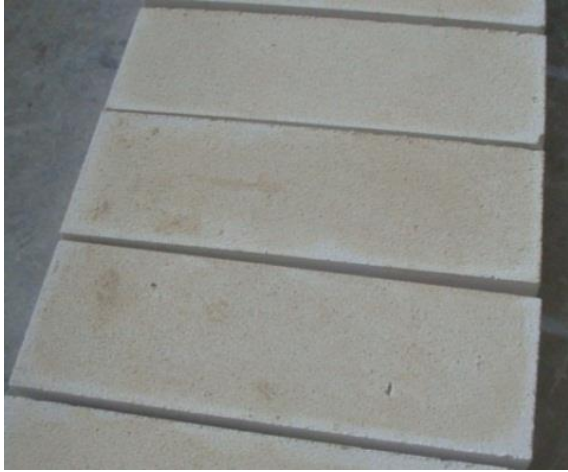
Fig. 1. The autoclaved aerated concrete with coated phase change material
