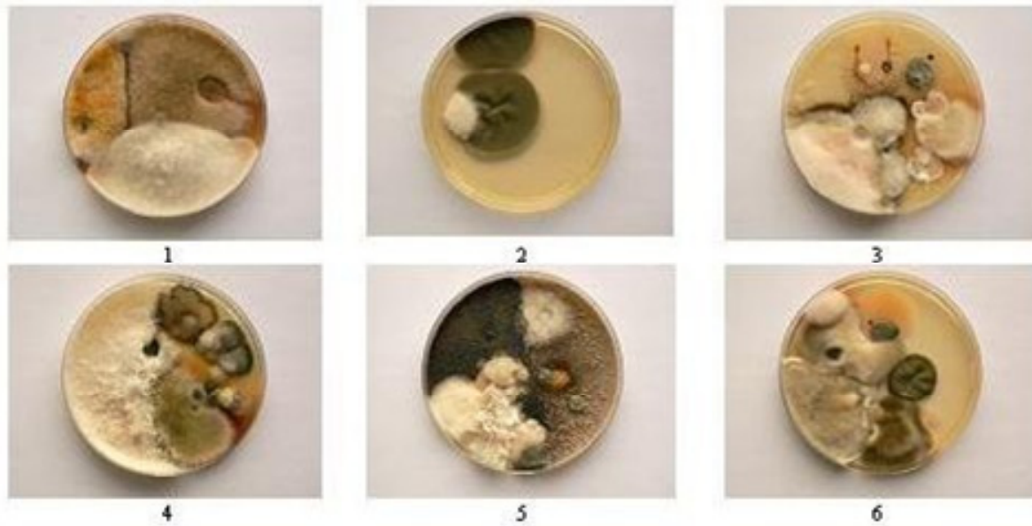
Fig. 1. Contamination with the propagules of fungi of steel plates coated with Zn chromated in different solutions after 1 year exposition to natural atmospheric conditions (Vilnius, Visoriai). Test solutions: 1. \text{Cr}(\text{NO}_3)_3 \cdot 9\text{H}_2\text{O} ; 2. \text{Cr}(\text{NO}_3)_3 \cdot 9\text{H}_2\text{O} + malonic acid; 3. Likonda 3Cr5; 4. Likonda 3CrV; 5. Likonda 3CrMC; 6. Likonda 3Cr5 + paste
