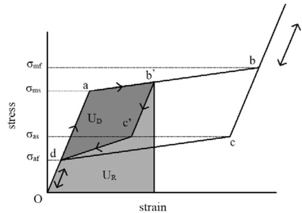
**Fig. 1.** Strain energy absorbed by SMA
