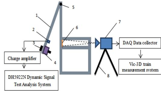
Fig. 2. Composite plate impact test schematic
