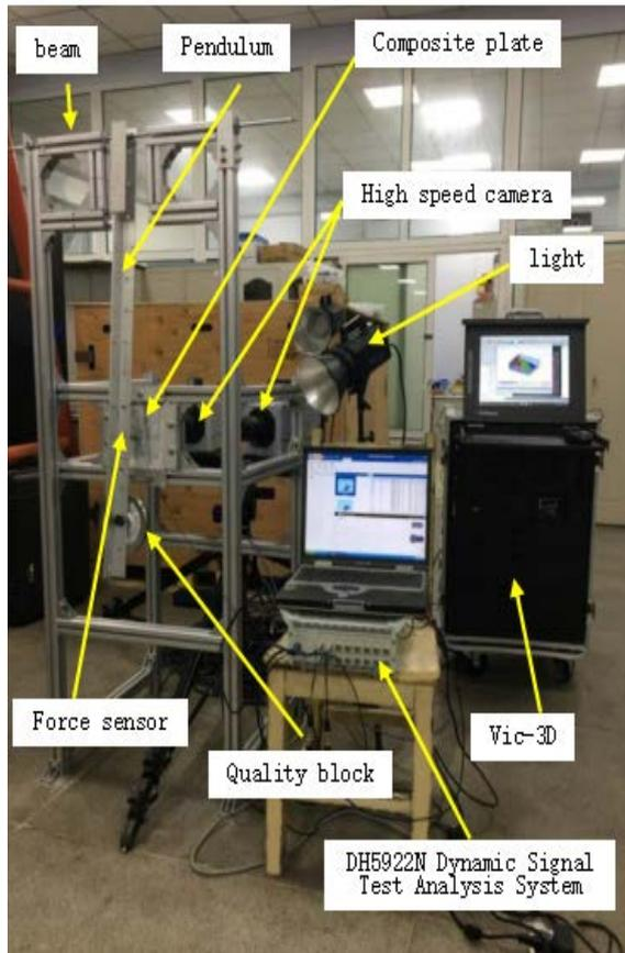
Fig. 3. Composite plate impact test bench
