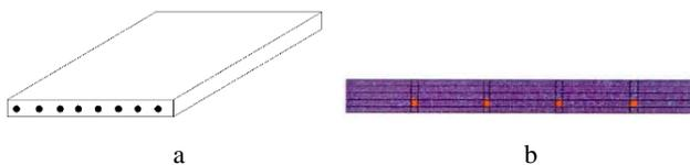
Fig. 4. Composite plate schematic: a–sketch map; b–specific laying position of SMA wire
