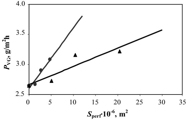
**Fig. 2.** Relation between the laminated leather water vapour permeability ( $P_{VG}$ ) and the perforation area  $S_{perf}$ :  $\bullet$  –  $\rho_1 = 0.83 \text{ cm}^{-2}$ ,  $\blacktriangle$  –  $\rho_2 = 3.64 \text{ cm}^{-2}$
