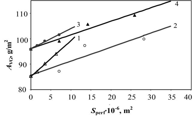
**Fig. 3.** Relation between the water vapour absorption  $A_{VG}$  and the perforation area  $S_{perf}$ :  $\Delta$  and  $\bullet$  –  $\rho_1 = 0.83 \text{ cm}^{-2}$ ,  $\blacktriangle$  –  $\rho_2 = 3.64 \text{ cm}^{-2}$  (1 and 2 – leather; 3 and 4 – laminated leather)
