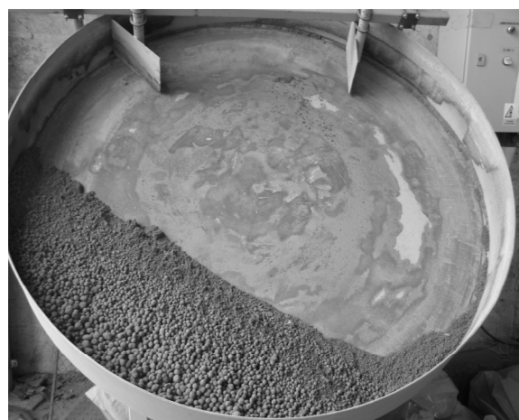
Fig. 11. First solidificates produced by S/S line pilot plant prototype
