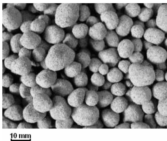
Fig. 10. First solidificates produced by S/S line prototype
