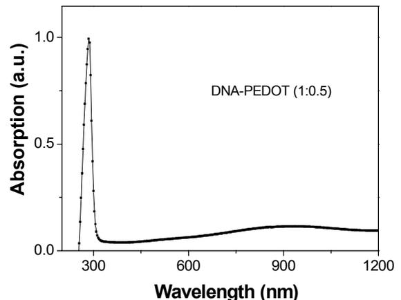
**Fig. 4.** Absorption spectrum of a DNA:PEDT-PSS (1:0.5) thin film
