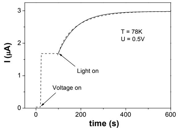
**Fig. 3.** Sample reaction on applied voltage pulse and white light pulse (dashed curve) as indicated on the Figure. The photocurrent growth could be approximated well by exponential dependence as indicated by the solid curve
