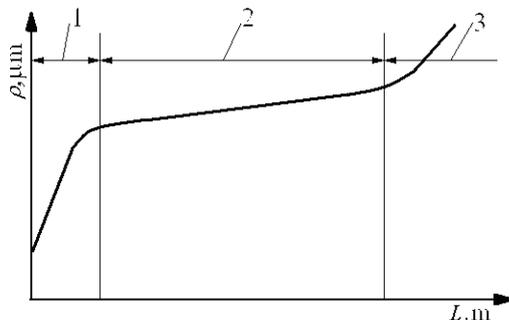
**Fig. 1.** The attrition process stages: 1 – initial; 2 – monotonic; 3 – emergency [2]
