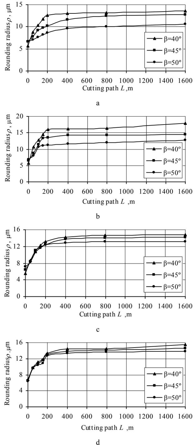
**Fig. 4.** Influence of the cutting path  $L$  on the rounding radius of the cutting edge  $\rho$ : a –  $u_z = 0.5 \text{ mm}$ ; b –  $u_z = 1.0 \text{ mm}$ ; c –  $u_z = 1.5 \text{ mm}$ ; d –  $u_z = 2.00 \text{ mm}$
