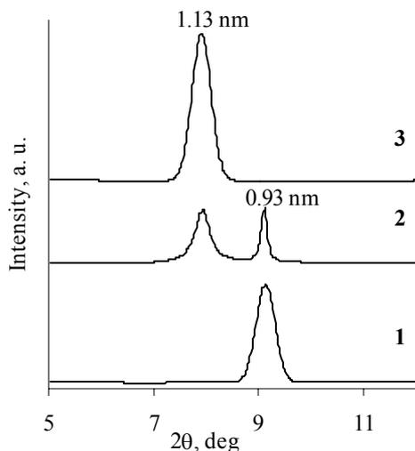
**Fig. 9.** Thermal type of tobermorite. XRD patterns after 3 h heating at 300 °C temperature. Duration of synthesis – 24 h and composition of initial mixtures: 1 – C/S=0.83, Na<sub>2</sub>O=0 %; 2 – C/(S+A)=0.83 ir A/(S+A)=0.025, Na<sub>2</sub>O=0 %, 3 – C/(S+A)=0.83 ir A/(S+A)=0.025, Na<sub>2</sub>O=5 %
