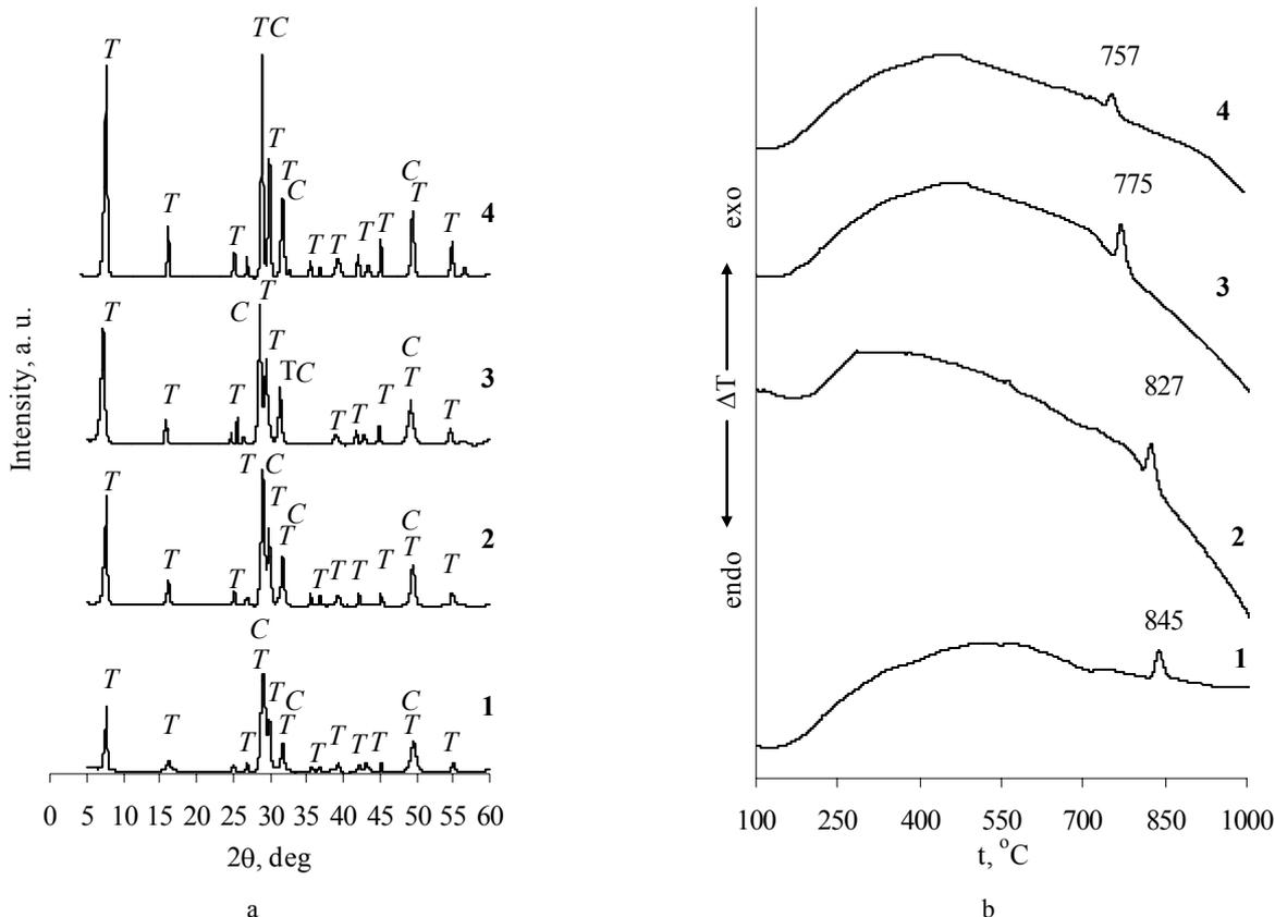
**Fig. 5.** XRD patterns (a) and DSC curves (b) of synthesis products from CaO and amorphous silica mixtures with  $\gamma\text{-Al}_2\text{O}_3$  additive when synthesis duration is 4 h. Amount of  $\text{Na}_2\text{O}$  added, %: 1 – 0; 2 – 1; 3 – 5; 4 – 10. Indexes: T – 1.13 nm tobermorite, C – C-S-H(I)
