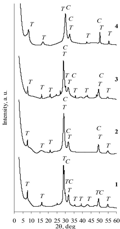
**Fig. 3.** XRD patterns of synthesis at 175 °C temperature products from CaO and SiO<sub>2</sub>·nH<sub>2</sub>O mixtures when duration of curing is 24 h and Na<sub>2</sub>O additive content, %: 1 – 0; 2 – 1; 3 – 5; 4 – 10. Indexes: T – 1.13 nm tobermorite, C – C-S-H(I)
