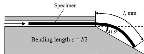
**Fig. 3.** Specimen bending in FAST system
