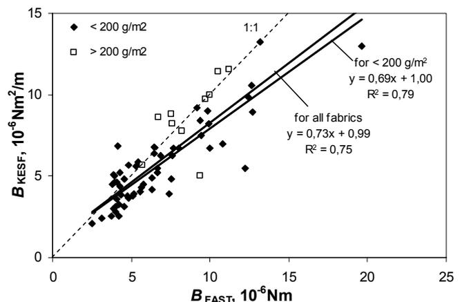
Fig. 11. The relationships between KES-F and FAST bending rigidity values for all analysed fabrics and light-weight (< 200 g/m<sup>2</sup>) fabrics
