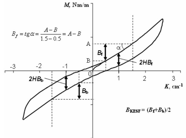
**Fig. 2.** Bending moment/curvature curve in KES-F system
