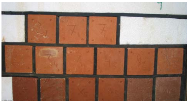
Fig. 5. Determination of frost resistance by one-side method of freezing-thawing
