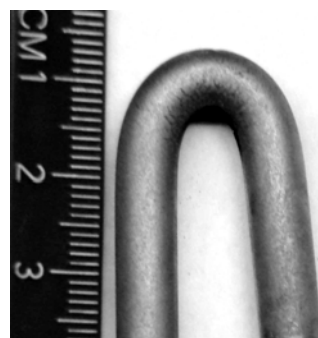
Fig. 12. Optical image of a coated by Co-W (28 at.%) and then folded Ø 6 mm Cu rod. Thickness of deposit ~50 µm, current density 30 mA/cm 2
