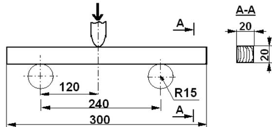
Fig. 1. Principal scheme of static bending test
