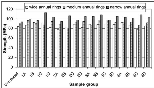
**Fig. 2.** Bending strength vs width of annual rings, heating duration (1, 2, 3, 4 is heating duration respectively 24, 48, 72 and 96 hours), and heating temperature (A, B, C, D is respectively 60, 80, 100 and 120 °C)
