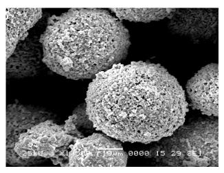
Fig. 1. Microstructure of WC-12%Co powder
