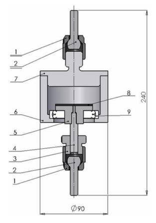
Fig. 2. The principal scheme of the adhesive strength device:
