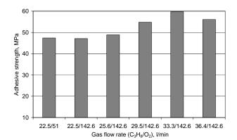
Fig. 7. Dependence of WC-12%Co coating, sprayed by MicroJet gun, adhesive strength on gas flow rate
