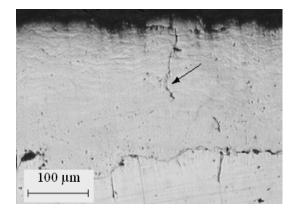
Fig. 4. Microstructure of the WC-12%Co coating sprayed by MicroJet gun at 36.4 l/min fuel gas supply rate
