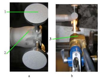
Fig. 3. Deposition of WC-12%Co coating on the specimens for determining adhesive strength: 1 – specimen; 2 – rotation device; 3 – spraying gun
