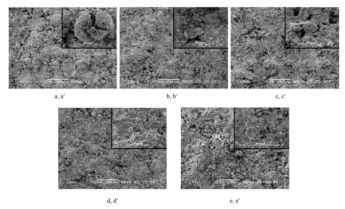
Fig. 6. Morphology of WC-12%Co coating sprayed by modified TopJet/2 gun at various gas ( $C_3H_8/O_2$ ) flow rates, l/min: a, b - 14.45/131; c, d - 21/131; e, f - 21.7/131; g, h - 27.4/131; k, l - 31.6/131 (marks size on selected parts a'-e' - 10  $\mu$ m)
