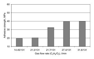
Fig. 8. Dependence of WC-12%Co coating, sprayed by modified TopJet/2 gun, adhesive strength on gas flow rate
