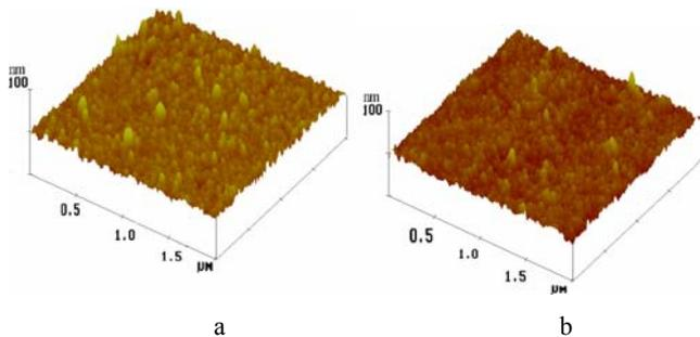
**Fig. 4.** AFM images of surface morphology of coatings obtained from sol: a – modified HMDS (0.25), b – HMDS (0.1)
