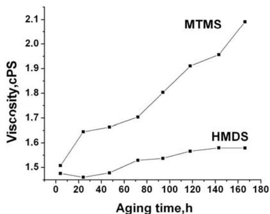
**Fig. 2.** Variation of viscosity with time of modified sol with MTMS (0.25) and HMDS (0.25) sol
