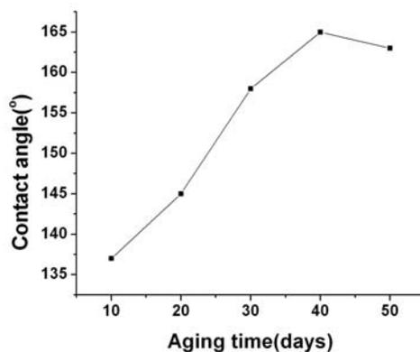
**Fig. 7.** Variation water contact angles with aging time for HMDS (0.25) modified silica coatings
