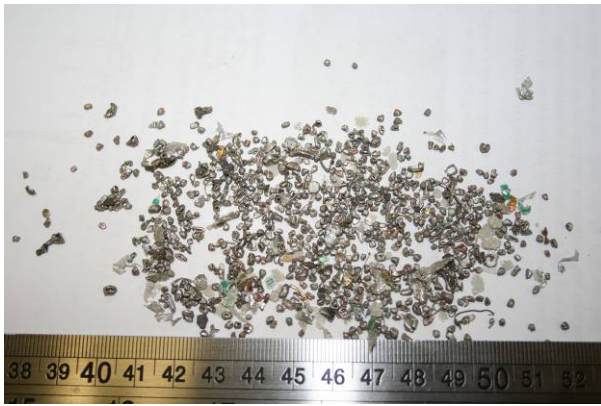
Fig. 6. Separated ferrous metals from the coarse fraction +1.25 – 2.5 mm
