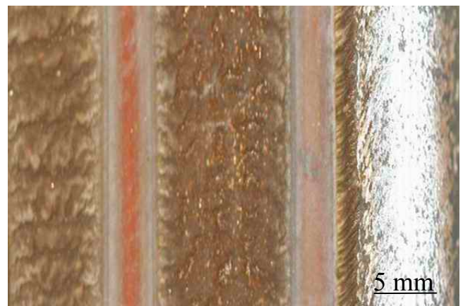
Fig. 3. The surface of laser beam treated steel Vanadis 6. Scan speed 300 mm/min, laser beam power 1000 W
