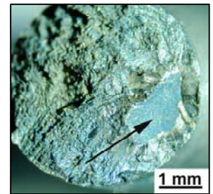
Fig. 9. Crystallographic crack initiation
