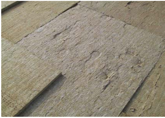
Fig. 2. Thermal insulation material (board in dimensions 2000 mm × 1200 mm) after walking on it
