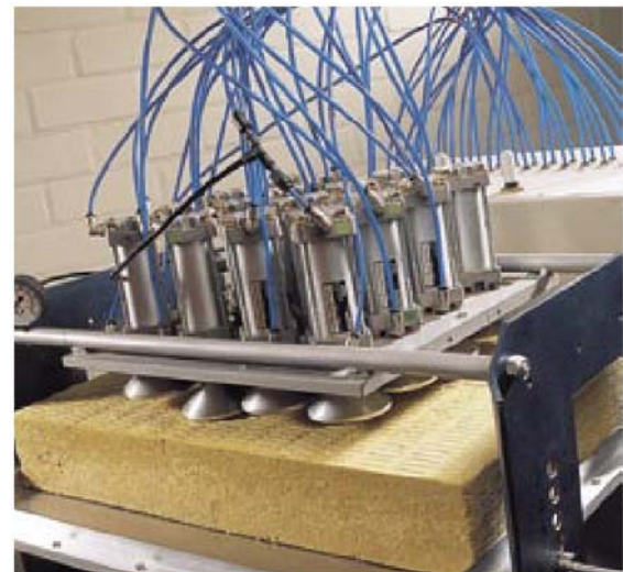
Fig. 4. Dynamic fatigue test on JW machine
