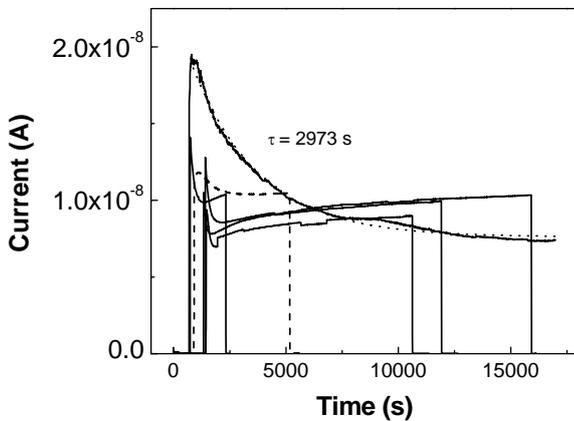
**Fig. 5.** Series of current transients measured at -20 °C after the onset of the light excitation corresponding to the photoconductivity maximum. Curves are shifted in time for the sake of convenience
