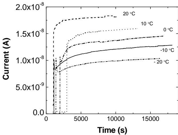
**Fig. 4.** Current transients measured at different temperatures, after the onset of the light excitation corresponding to the photoconductivity maximum. Curves are shifted in time for the sake of convenience
