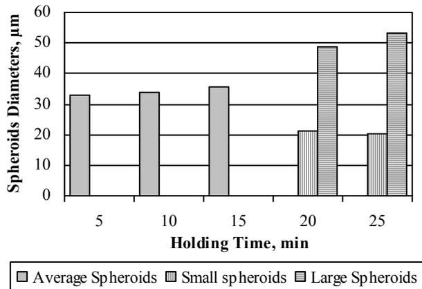
Fig. 3. Size of the graphite spheroids diameters in 10 mm thick plates as a function of the time after spheroidizing treatment
