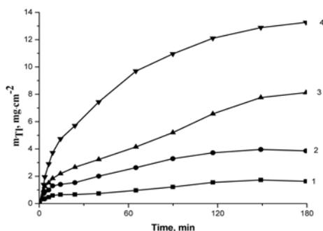
**Fig. 3.** Dependence of the content of thallium in sulphide layer on PE film on sulphurization time under treatment it with solutions of  $\text{H}_2\text{S}_{33}\text{O}_6$  for different periods of time. The period of treatment with 0.1 M  $\text{Tl}_2\text{SO}_4$  solution at 80 °C was 10 min. The temperature (°C) of  $\text{H}_2\text{S}_{33}\text{O}_6$  solution: 1–25, 2–40, 3–60, 4–80
