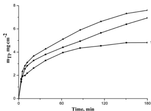
**Fig. 5.** Dependence of thallium content in sulphide layer on PE film on sulphurization time under treatment it with solution of  $\text{H}_2\text{S}_{33}\text{O}_6$  at 60 °C for different periods of time. The period of treatment with 0.1 M  $\text{Tl}_2\text{SO}_4$  solution at 80 °C was 10 min. The concentration ( $\text{mol}\cdot\text{dm}^{-3}$ ) of  $\text{Tl}_2\text{SO}_4$  solution: 1–0.001, 2–0.05, 3–0.1
