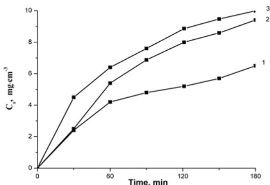
**Fig. 1.** Dependence of the content of sulphur in layer on PE film on sulphurization time under treatment it with solutions of  $H_2S_nO_6$  at  $60^\circ C$ . The average number of sulphur number atoms ( $n$ ) in polythionic acid molecule: 1–21; 2–33; 3–45
