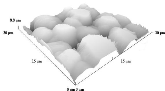
**Fig. 11.** AFM image of Tl<sub>x</sub>S<sub>y</sub> films on polyethylene. PE initially treated with a solution of H<sub>2</sub>S<sub>33</sub>O<sub>6</sub> at 60 °C for 120 min and then immersed in Tl<sub>2</sub>SO<sub>4</sub> solution at 80 °C for 10 min
