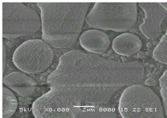
**Fig. 10.** SEM image of Tl<sub>x</sub>S<sub>y</sub> films on polyethylene. Image area (16×10) µm<sup>2</sup>
