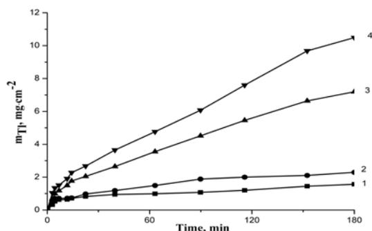
**Fig. 7.** Dependence of thallium content in sulphide layer on PE film on sulphurization time under treatment it with solution of  $H_2S_{33}O_6$  at 60 °C for different periods of time. The sulphured PE treated with 0.1 M  $Tl_2SO_4$  solution at 80 °C. Duration (min) of sulphured PE treatment with  $Tl_2SO_4$  solution: 1–2, 2–5, 3–10, 4–20
