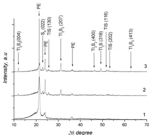
**Fig. 9.** X-ray diffraction patterns of thallium sulphide layers on the surface of PE. PE initially treated with a solution of H<sub>2</sub>S<sub>33</sub>O<sub>6</sub> at 80 °C for different times and then immersed in Tl<sub>2</sub>SO<sub>4</sub> solution at 80 °C for 10 min. Sulphurisation time (min): 1–15, 2–60, 3–120
