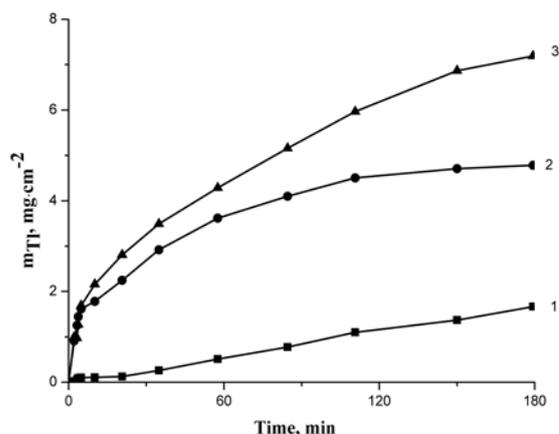
**Fig. 4.** Dependence of thallium content in sulphide layer on PE film on sulphurization time under treatment it with solution of  $\text{H}_2\text{S}_{33}\text{O}_6$  at 60 °C for different periods of time. The period of treatment with 0.1 M  $\text{Tl}_2\text{SO}_4$  solution was 10 min. The temperature (°C) of  $\text{Tl}_2\text{SO}_4$  solution: 1–40, 2–60, 3–80
