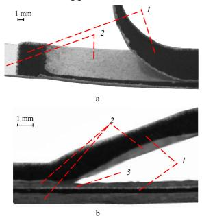
Fig. 4. Photo of a glued (glue Eukalin) flocked sample made from 1 mm-length Capron flock and paperboard Duoplex UD-3, after breaking off: a – view from the top; b – section view; 1 – flock coating; 2 – paperboard; 3 – glue layer
