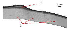
Fig. 8. Photo of a glued (glue Eukalin) flocked sample made from 1 mm-length Capron flock and paperboard Arktika GC-1, after breaking off: 1 – inner delamination; 2 – warping
