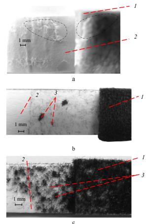
Fig. 3. Photo of the glued (glue Eukalin) flocked samples with a flock coating on paperboard: Arktika GC-1 after breaking off: a – 0.5 mm-length Capron; b – 0.75 mm-length viscose; c – 1.0 mm-length Capron: 1 – flock-coating (face side); 2 – paperboard (reverse side of flocked packaging); 3 – broken-off flock fibres
