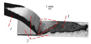
Fig. 5. Photo of a glued (glue Eukalin) flocked sample made from 1 mm-length Capron flock and paperboard Arktika GC-1, after breaking off: 1 – flock coating; 2 – paperboard; 3 – broken off flock coating
