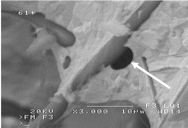
**Fig. 10.** Hydrogen blister formed at the composite reinforcement fibre
