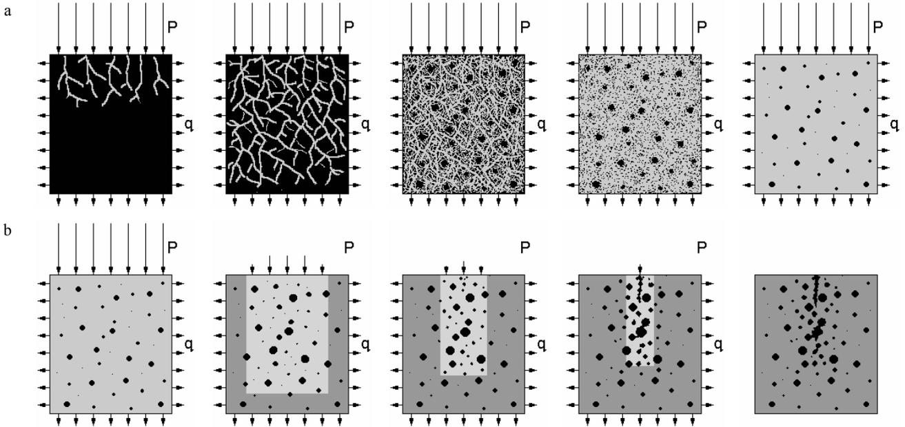
**Fig. 2.** A scheme of porosity formation in a composite casting with saturated reinforcement [7, 8]; a – the stage of reinforcement saturation; b – the stage of cooling and solidification of the composite matrix
