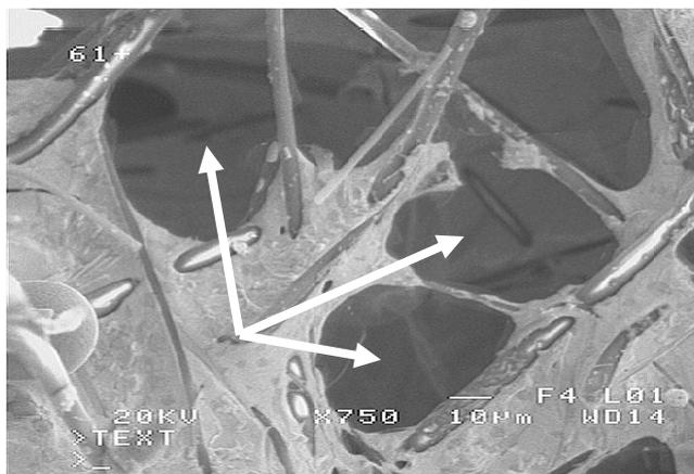
**Fig. 8.** Gas miniocclusions trapped between the composite reinforcement fibres
