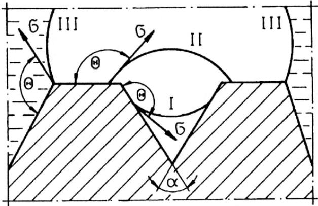
Fig. 4. Diagram of heterogeneous nucleation and growth of blisters
