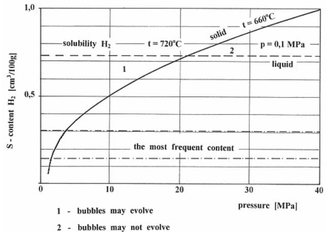
**Fig. 3.** Possibility of hydrogen desorption from liquid aluminum as a function of pressure: 1 – the desorption condition is met and the blisters may release; 2 – the desorption condition is not met and the blisters can not release
