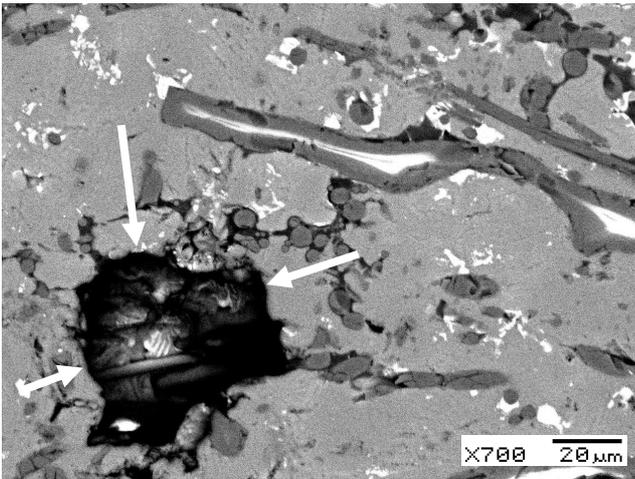
**Fig. 11.** Large gas occlusion with clear decompression features (magnification 700×)
