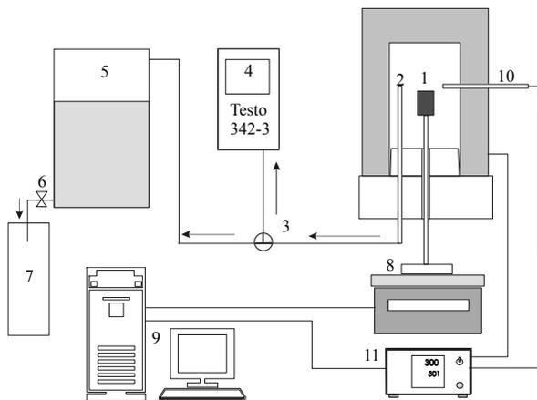
**Fig. 1.** A system of furnace control and gas off take: 1 – furnace muffle with a specimen, 2 – gas off take pipe, 3 – three-way valve, 4 – gas analyser, 5 – sealed water container, 6 – valve, 7 – measuring cylinder, 8 – scales, 9 – computer, 10 – thermocouple, 11 – temperature regulator
