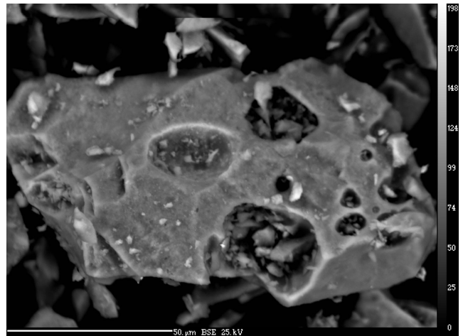
Fig. 12. SEM micrograph of K-Na-Al-Si-O precursor gel annealed at 750 °C for 5 h
