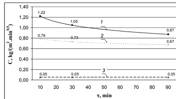
**Fig. 3.** The impact of time of impregnation on coefficient of water adsorption due to capillary action in the silicate samples: 1 – silicate block ( $\rho = 1740$  kg/m<sup>3</sup>); 2, 3 – split face brick,  $\rho = 1870$  kg/m<sup>3</sup>: 2 – not hydrophobized, 3 – hydrophobized
