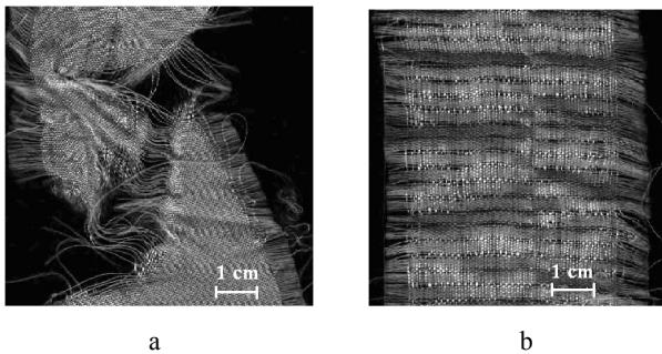
**Fig. 2.** The views of break: a – weaves, the floats of which are evenly distributed within the whole area of the woven fabric; b – across striped weaves
