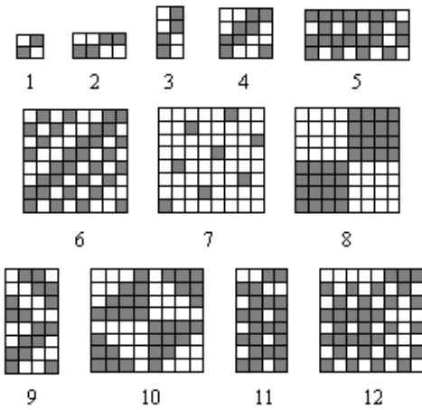
**Fig. 1.** The weaves used in experiment: 1 – plain weave ( $P_1 = 1$ ); 2 – weft rib ( $P_1 = 1$ ); 3 – warp rib ( $P_1 = 1.31$ ); 4 – twill 2/2 ( $P_1 = 1.26$ ); 5 – weft direction Bedford cord ( $P_1 = 1.27$ ); 6 – fancy twill ( $P_1 = 1.11$ ); 7 – sateen ( $P_1 = 1.79$ ); 8 – basket weave ( $P_1 = 1.88$ ); 9 – broken twill ( $P_1 = 1.18$ ); 10 – crape weave ( $P_1 = 1.41$ ); 11 – warp direction Bedford cord ( $P_1 = 1.18$ ); 12 – mock leno ( $P_1 = 1.12$ )
