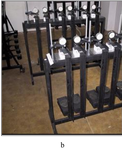
Fig. 1. The schematic of the device for determining the creep strains of expanded polystyrene (EPS) a): 1 – dial gauge; 2 – loading suspension; 3 – movable plate for uniform distribution of loading; 4 – test sample; 5 – support beam; 6 – invariable load; b) a general view of the device for test
