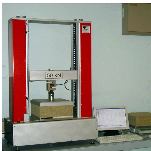
Fig. 2. Testing machine for compression “UTC 50 kN”
