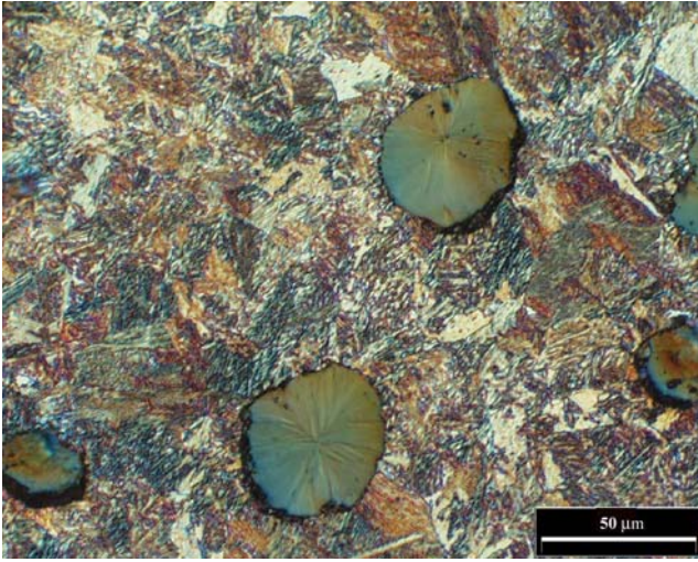
Fig. 2. Structure of ADI transformed during 40 minutes at 400 °C. (Nital etching, the Nomarski method, actual magnification 375×)
