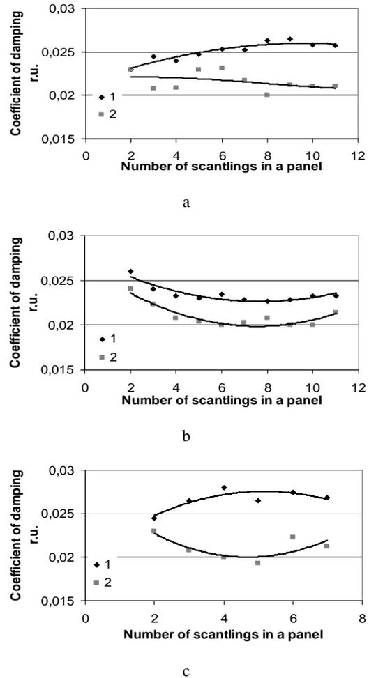
**Fig. 4.** Variation of panel coefficient of damping depending on the number of scantlings in the panel (panel width): a – gluing up scantlings with close values of coefficient of damping; b – gluing up scantlings with more different values of the coefficient of damping; c – gluing up scantlings with highly different coefficients of damping; 1 – mean coefficient of damping of the used scantlings, 2 – panel coefficient of damping
