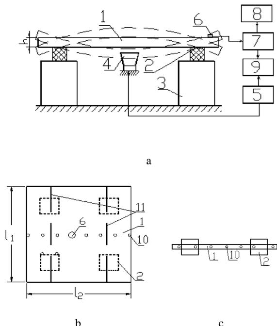
**Fig. 1.** Study stand (a) of wooden articles and location scheme of vibration measurement points in the case of plate (b) and beam (c): 1 – wooden assortment and its bend form (dashed line); 2 – elastic elements; 3 – massive supports; 4 – acoustic vibrator; 5 – generator of electric vibrations; 6 – transducer; 7 – measuring device; 8 – oscilloscope; 9 – phase-meter; 10 – fastening points of transducer; 11 – vibration lines of the first bend forms (modes) in longitudinal direction
