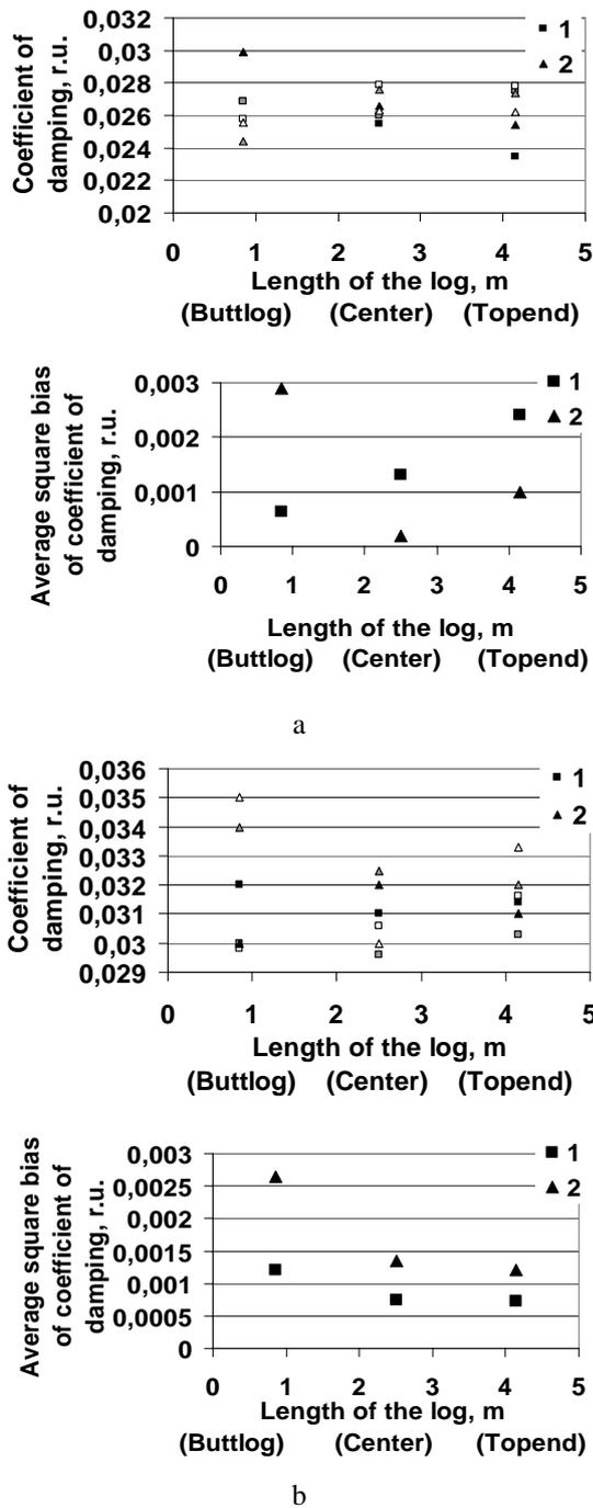
**Fig. 3.** The regularities of coefficient of damping distribution in an oak log and average square bias of coefficient of damping: a – along the grain; b – across the grain; where 1 – in central boards, 2 – in side boards
