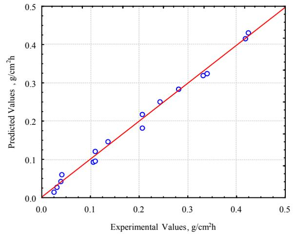
**Fig. 8.** Comparison of the experimental and the calculated values of capillary rate of the mass flow under vacuum in the direction of freezing
