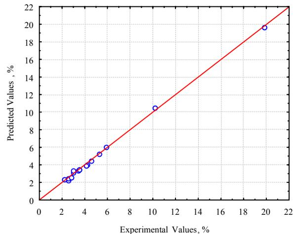
**Fig. 4.** Comparison of the experimental and the calculated values of relative wall thickness of the pores and capillaries
