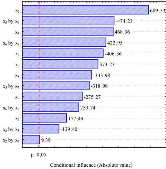
**Fig. 11.** Conditional influence of technological factors on capillary rate of the mass flow in the direction of freezing
