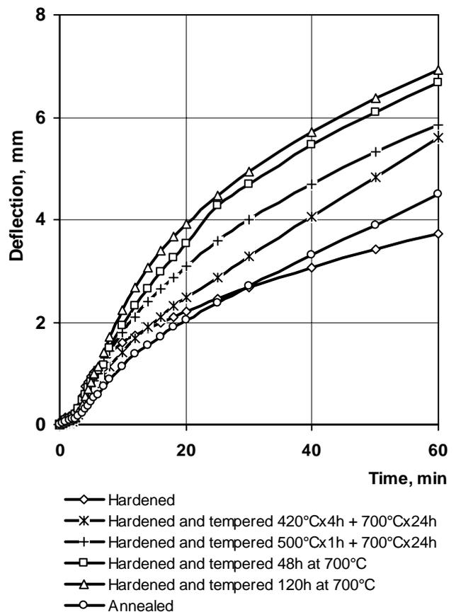
Fig. 6. Dependence of steel 14X17H2 plasticity on structural state during tempering at 650 °C temperature. Bending stress 90 N/mm<sup>2</sup>
