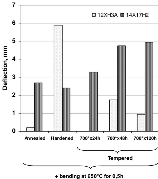
Fig. 4. Influence of structural state of steel on plasticity during tempering at 650 °C. Bending stress 90 N/mm<sup>2</sup>
