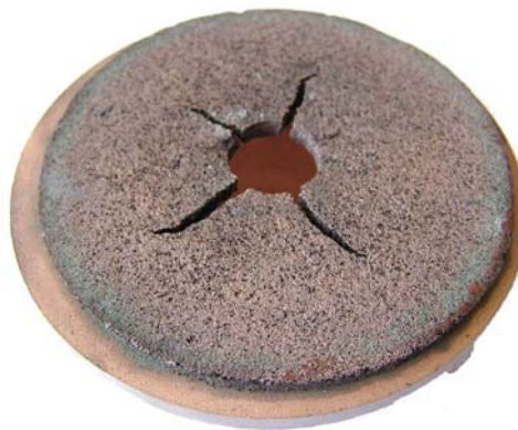
Fig. 6. The presence of residuals of the infiltrant in infiltration of Fe-C with copper. Diameter of details – 80 mm
