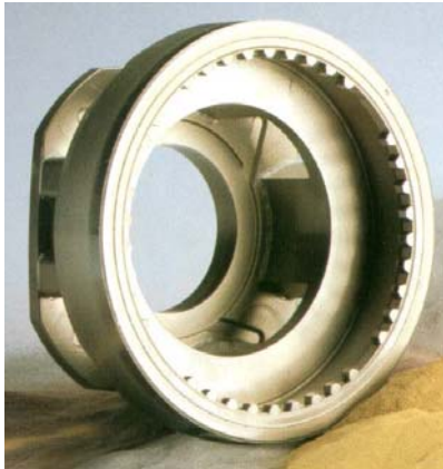
Fig. 2. Use of brazing in manufacture of a conveyor component [9]
