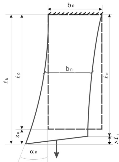
**Fig. 3.** Specimen's shape after stretching and measured parameters
