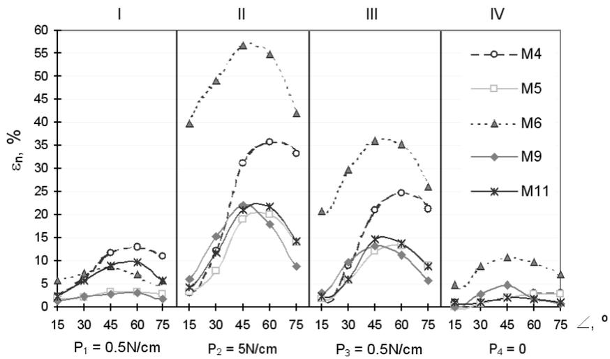
Fig. 4. The influence of loading conditions (I, II, III and IV stages) and cut directions of specimen upon the elongation  $\varepsilon_n$
